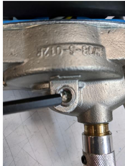
(Figure 3) Air Lock Relief Valve
